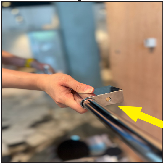
Step 8: Attach the shower rod to the wall bracket until it clicks securely into place
