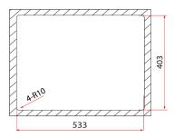
\* Measured in Millimeters (mm)
