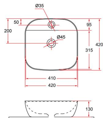
\* Measured in Millimeters (mm)
